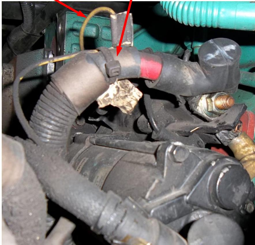
The Switch lead must be re-routed from top to the bottom of the starter, as the new M96R3019SE Switch connection is at the bottom of the starter motor.
